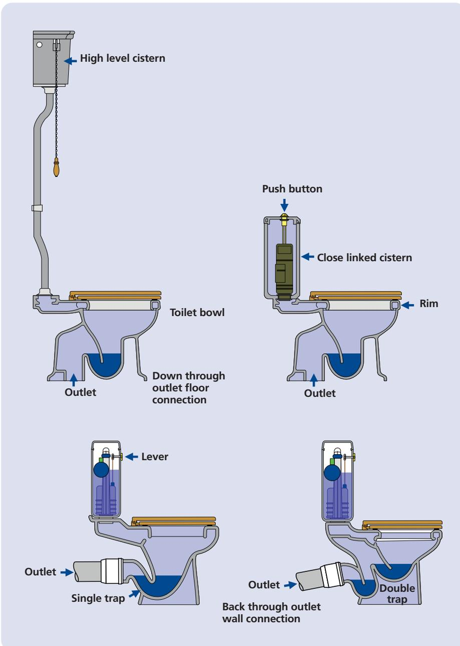
If the water takes a long time to drain out of the toilet bowl, or the water is rising towards the rim, this is a sign that your toilet has a blockage in the soil pipe. You need to urgently find the cause of the blockage before it becomes unusable.
